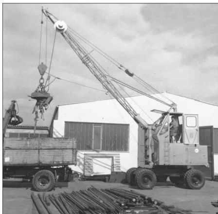
1962: rope-driven S833 with elevated operator cab
